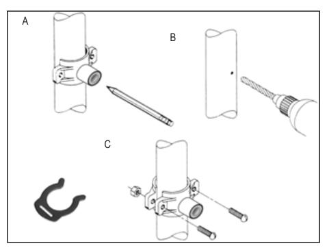
Figure 11: Drain Saddle Assembly
